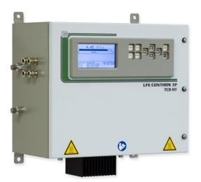
The high temperature version includes the complete thermostat control of the TCD detector as well as all gas paths and connectors within the analyzer for temperatures above the sample gas dew-point in conjunction with external heated gas lines for gas inlet and gas outlet.
